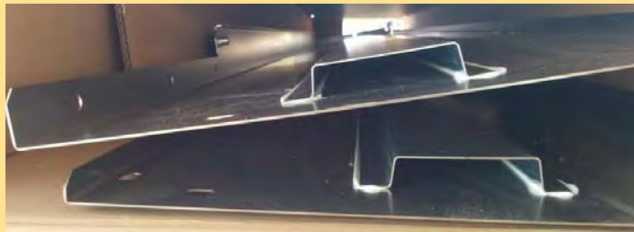
Stiffeners at the back of car body panels
