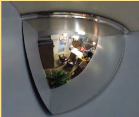
Dome corner mirror inside elevator for wheelchair reversing; source: Safety-Security-Mirrors
