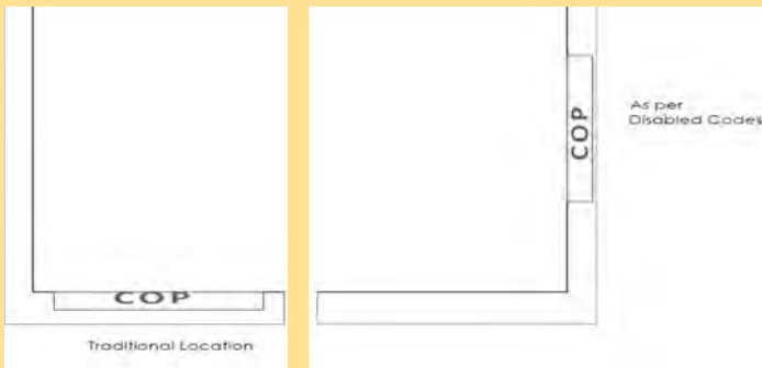
Location of COP, complying with accessibility code EN 81-70
